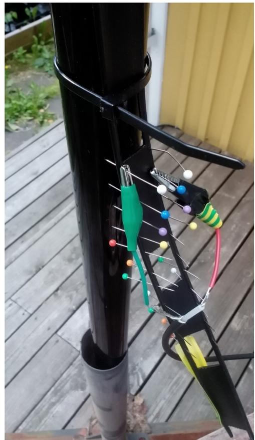
point – or one third up the cable. I actually found my best point in terms of the lowest SWR and the nearest resonance to 28.5MHz to be a 6cm notch 2.31m up from the bottom.
